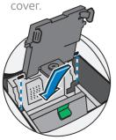
4.4 Slide the print head pegs down into the grooves.
