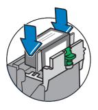
4.7 Insert the cartridge. The ridges on the cartridge slide into the grooves.
