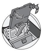
4E. Push the printhead back into place. You should hear a click when it is seated correctly.
