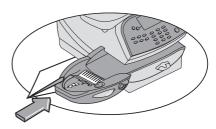
Position the envelope or tape sheet against the registration wall of the system and slide it to the right until the system grasps it. The system prints the digital meter stamp and ejects the envelope/tape sheet.
