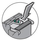
8. Close the top cover. The system automatically recognises the new cartridge and in a few moments returns you to the Home screen.
