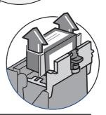
**NOTE:** If you are NOT changing the printhead, skip to Step 5. If you have been directed by a representative of your machine supplier to change the Print Head, continue with step 4A below.
