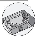
4B. While squeezing, lift and tilt to the right the printhead. The printhead should come up out of the machine.
