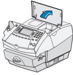
5.1 When the display asks you to install the Print Head, open the top cover.
