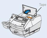
3.1 Open ink access cover and remove tape and shipping material.
