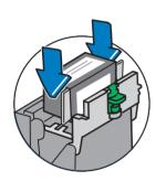
5.7 Insert the cartridge. The ridges on the cartridge slide into the grooves.
