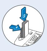
3.4 Push the tape lever to the right and drop tapes into the slot. The printable side of the tape should be facing towards the right.
