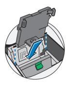
5.4 Slide the print head pegs down into the grooves.
