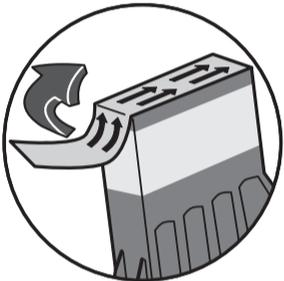
5.3 Open the packaging for the ink cartridge and take off the protective tape from the bottom.
