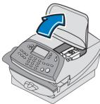
4.1 When the display shows 'Print head not detected. Open cover to install print head and ink tank', open the top cover.
