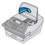
4.9 Close the top cover. The franking machine will now go through a setup cycle which takes up to 2 minutes.
