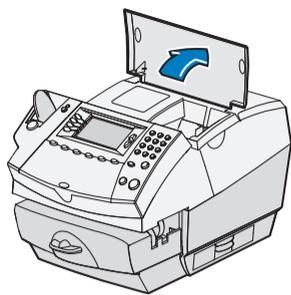
5.1 When the display asks you to install the Print Head, open the top cover.
