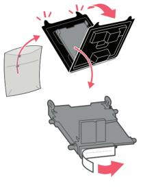
c. Unwrap the Printhead and remove the protective strip.
