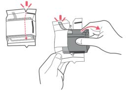
e. Keep squeezing the tabs and push the Printhead flat against the and make sure you remove the wall. The tabs will click open when silver foil strip. placed correctly.
